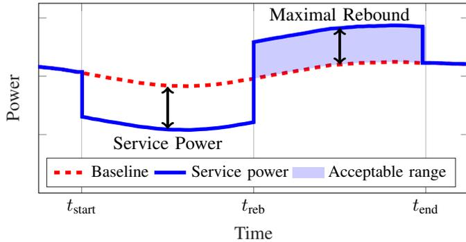
Fig. 2. Sketch of a relative DSO-service request.
