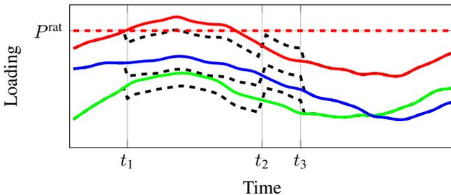
Fig. 10. Sketch of a scheduled load reduction - blue, red and green lines depict load scenarios, the black line represents a load reduction service
