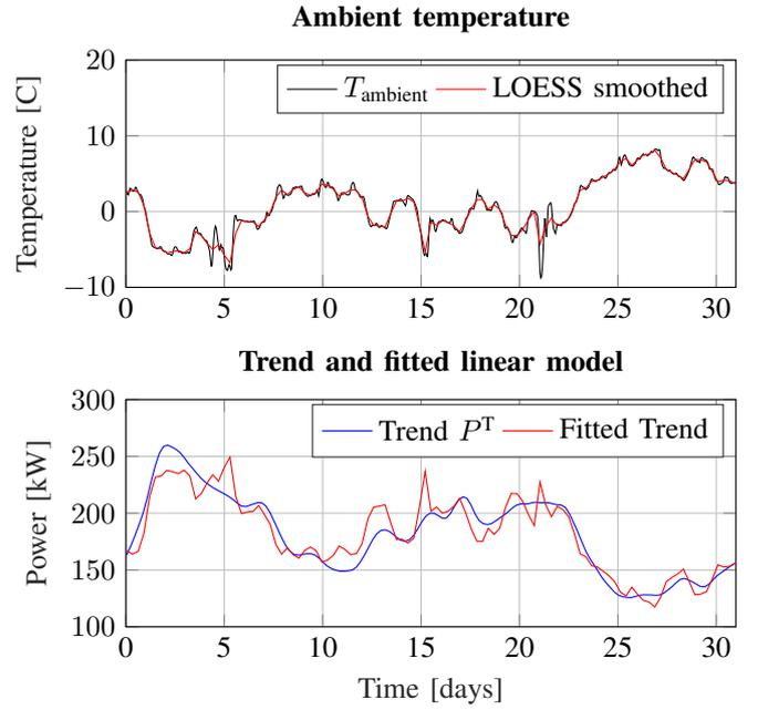
Fig. 6. Top: Ambient temperature of January 2016. Bottom plot depicts trend  $P^T$  for January (blue) together with the fitted linear function of the ambient temperature (red).
