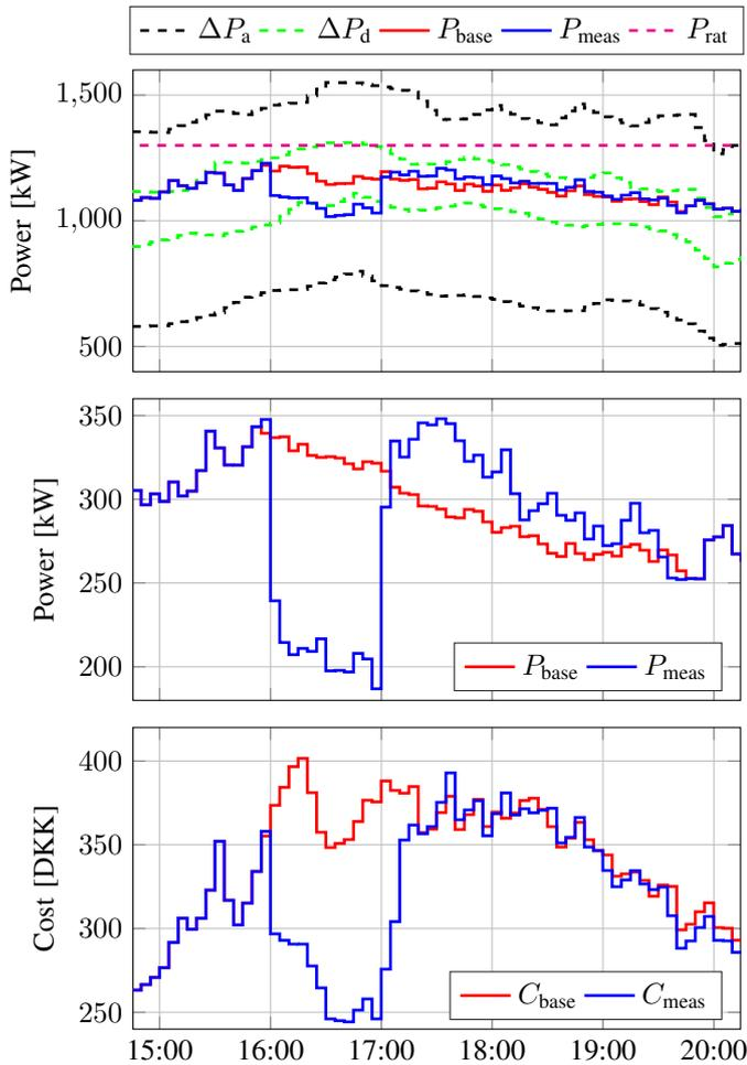
Fig. 13. DSO service delivery on the 25th of January 2019. Top: power flow on transformer station, middle: aggregated DER power consumption, bottom: modelled cost of transformer loading
