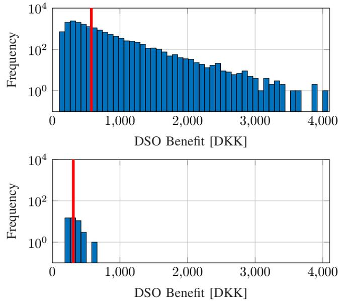
Fig. 16. Logarithmic histogram of service benefit for DSO service at time of request (top) and activation (bottom).
