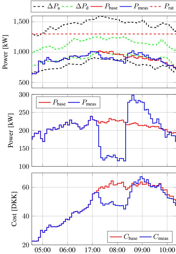
Fig. 15. DSO service delivery on the 22nd of February 2019. Top: power flow on transformer station, middle: aggregated DER power consumption, bottom: modelled cost of transformer loading
