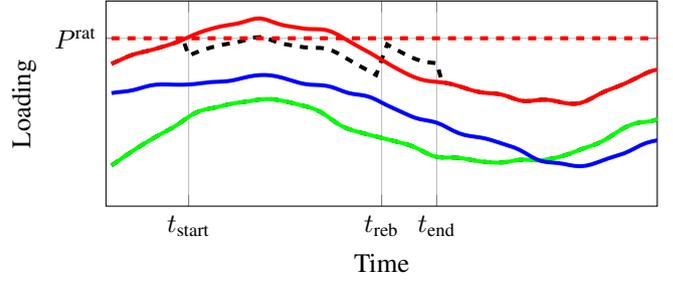
Fig. 11. Sketch of a conditional load reduction - blue, red and green lines depict load scenarios, the black dashed line represents a load reduction service
