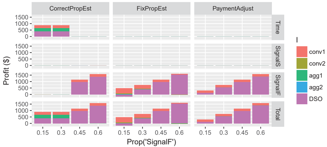
Figure 36: MIP upper bound LP price: Profit of each aggregator and the DSO service provider. FixPropEst assumes that agents bid and are paid assuming \mathbb{P}_{SignalF}=0.45 and do not receive (or pay) an adjustment for being dispatched more or less than 0.45 \cdot L days. PaymentAdjust adjusts the payment to each agent using the equations in sub-sub section 2.4.3.
