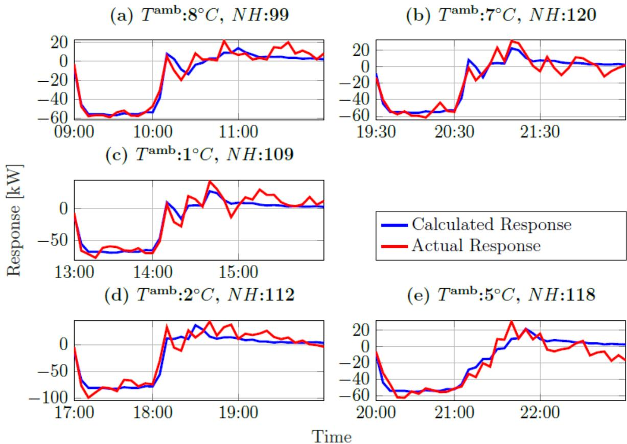
Figure 6: Test results from rebound validation
