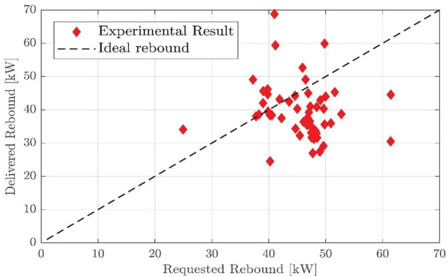
**Figure 9: Delivered vs requested rebound for TSO services during HS3**
