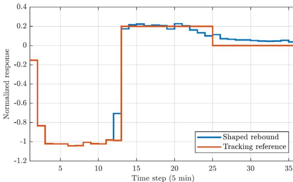
Figure 3: Shaped rebound behaviour for a 60 minutes rebound block
