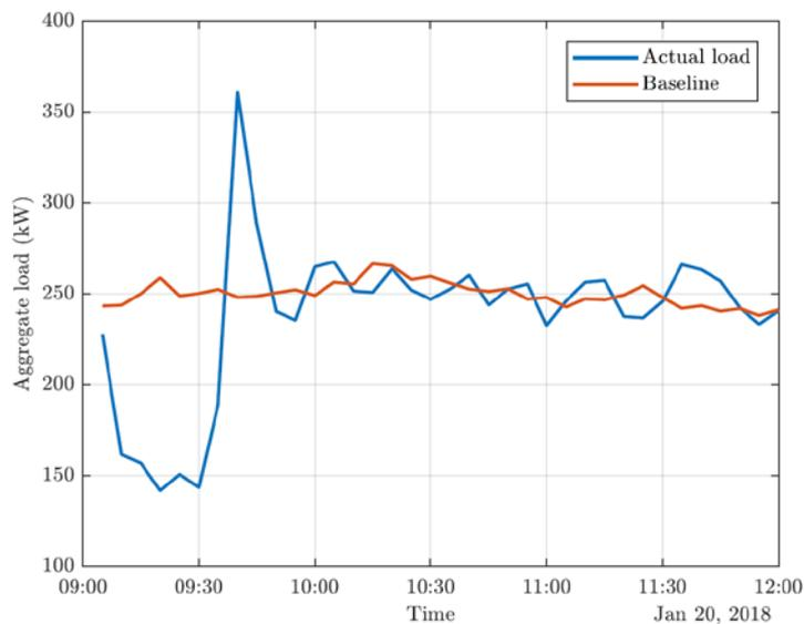
Figure 1: Effect of communication delay on the load response
