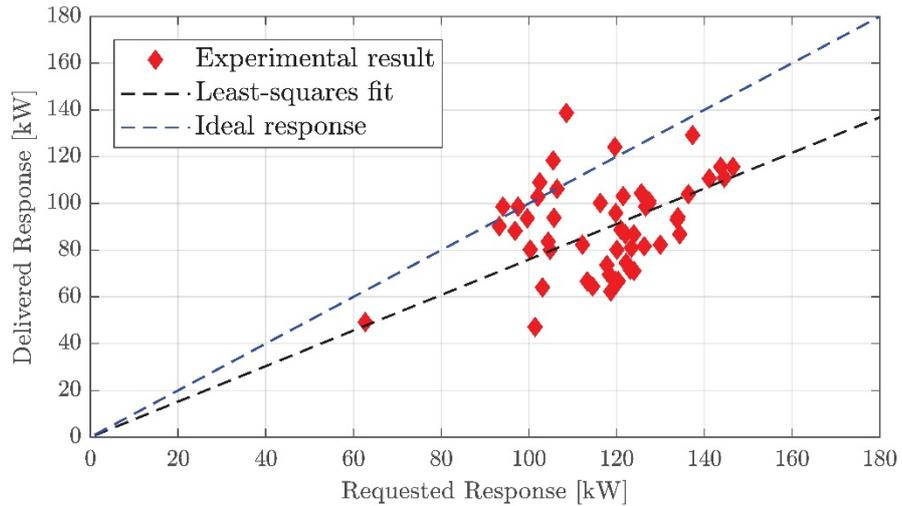
**Figure 8: Delivered vs requested response for TSO services during HS3**
