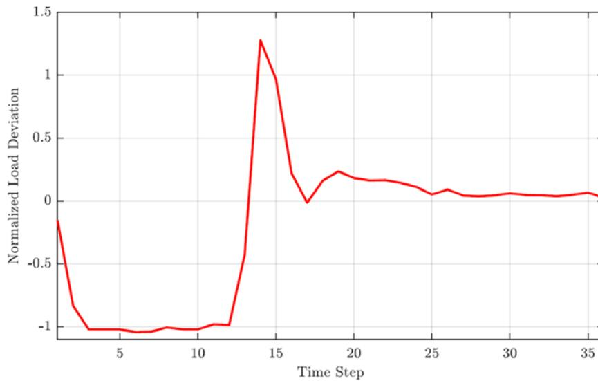
**Figure 2: Averaged normalized response and rebound for 60 min tests, in the uncontrolled rebound case [the duration of each time step is equal to 15 min].**
