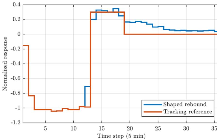
Figure 5: Shaped rebound behaviour for a 30 minutes rebound block
