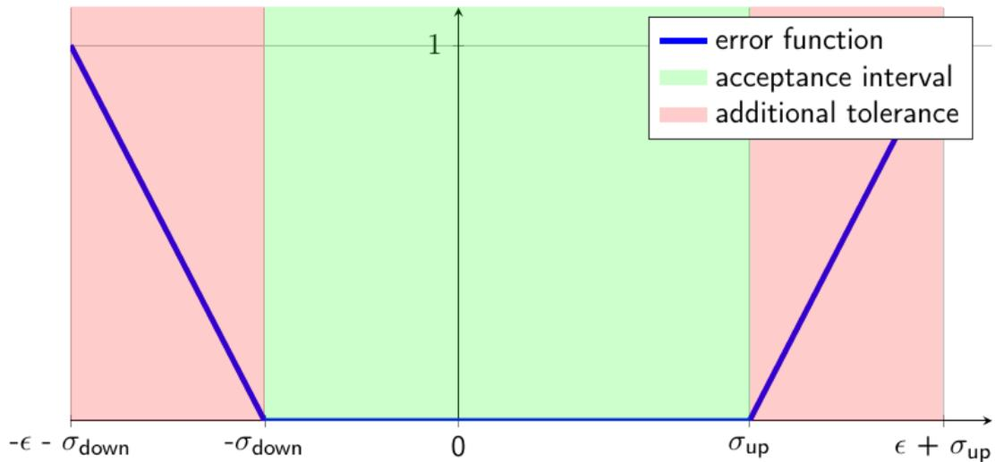
Figure 2: Error function  $f(x)$  mapping the deviation from the ideal response to a performance value
