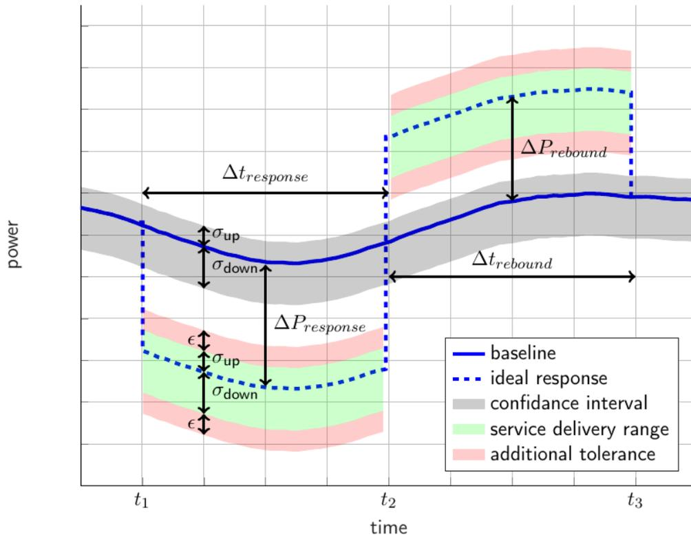
**Figure 2: Sketch of a load reduction service with rebound showing confidence interval, acceptable power interval during service delivery and the additional tolerance**
