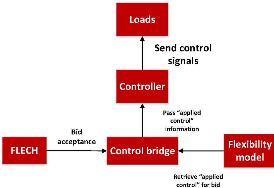
Figure 5: Use of the flexibility model for delivering a service
